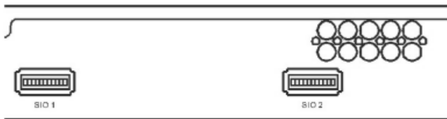
Figure 3- 5. SIO 1 and SIO 2 Stacking ports at the rear of the AT-9724TS
